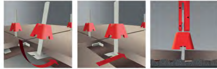
Position strap and cap Lay the tile Attach setting tool
