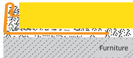
■ Cross-sectional image of a Schlüter®-Schiene-E profile
