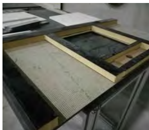
Reinforcements with expanded Polyurethane
